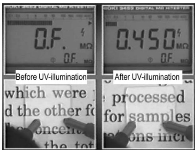
Fig. 7 Photoinduced conduction in H - -loaded C12A7 thin films. Both electrically insulating (lower left) and conductive (lower right) films appear colorless and transparent. The scales in the images show the electrical conductivity of each film
